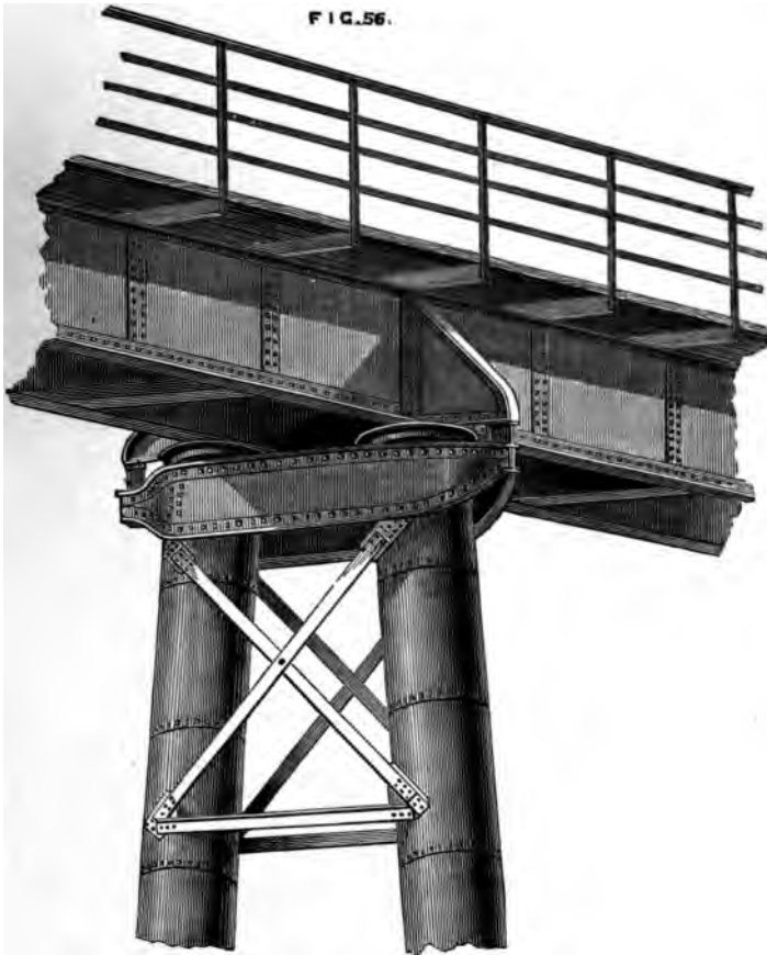
Fig. 56 shows the top of one of the piers, with a portion of the main girder, attachments, bracing, &c. A cast-iron bed-plate is interposed between the con-
